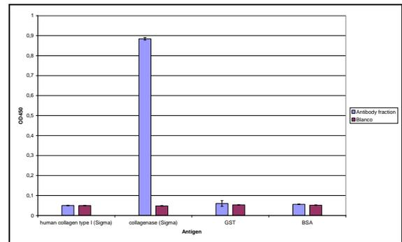
Figure 1: Specificity of Anti-Collagenase from *clostridium histolyticum* (Sigma-Aldrich, C0773) Immunoglobulin, clone 1D2, determined by ELISA. Antibody fraction (0.75 mg/ml) 700X diluted in PBS containing 0,05% tween-20 and 5% non fat dry milk. Antibody was tested on various recombinant protein substrates i.e. Human type I collagen (Sigma-Aldrich, C5483), GST (pGEX-2T) and BSA, 98% (Sigma).
